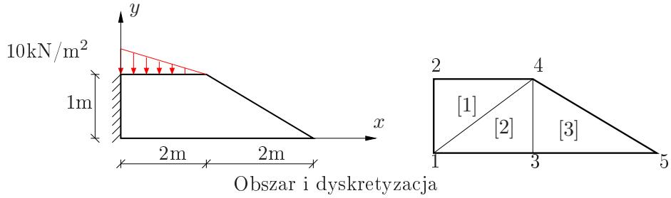
$$P_i^{(e)} = \int_{\partial e \cap \partial \Omega_N} \mathbf{N}_i \cdot \hat{\mathbf{t}} \, ds, \quad \hat{\mathbf{t}} = \begin{pmatrix} 0 \\ 5x - 10 \end{pmatrix}, \quad x \in [0, 2], \quad y = 1$$
