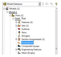
Mark heat\_flux area, press button Done, next Use Default Orientations or Other Method and then in window Edit Material Orientation press button OK.
