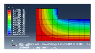
Remember about checking temperature in the same point as for mesh1. Results for second mesh:
