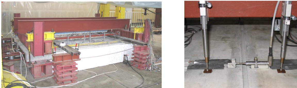
Fig. 1 Test setup and the view of joint between slab elements.
