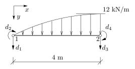
**Problem 3.** Use the FEM algorithm to solve the beam shown, i.e. calculate the vectors of nodal displacements and reactions, and make diagrams of cross-section force distributions.
