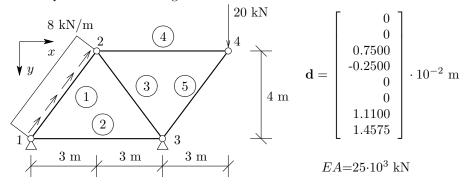
**Problem 9.** Determine the right-hand side vector in FEM equation set for the frame shown.
