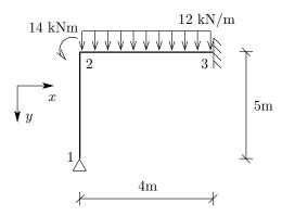
**Problem 10.** Present in a graphical manner the assembly of stiffness matrices for elements 2 and 3 of the frame shown below. Determine the global right-hand side vector  $\mathbf{f}$  in FEM equation set.
