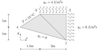
**Problem 2.** Calculate the heat flux density vector  $\boldsymbol{q}$  and temperature at point A(1.0,1.5) of the configuration discretized using 1 finite element. The input data contain: dof vector  $\boldsymbol{\theta}$ , conductivity matrix  $\mathbf{k}$  and shape functions.
